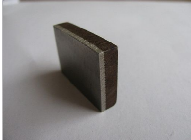
--Explosive bonding-- (Zigzag joint surface)
